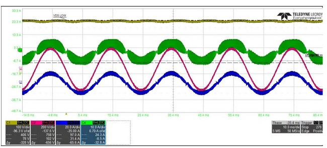
Figure 41 Steady-state waveforms at 230 V, 50 Hz AC voltage, 50 percent load
