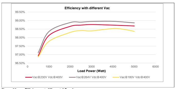
Figure 38 Efficiency at different AC voltage
