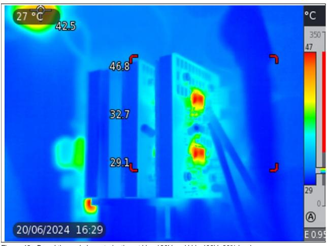
Figure 46 Board thermal characterization at Vac 180V and Vdc 400V, 60% load
