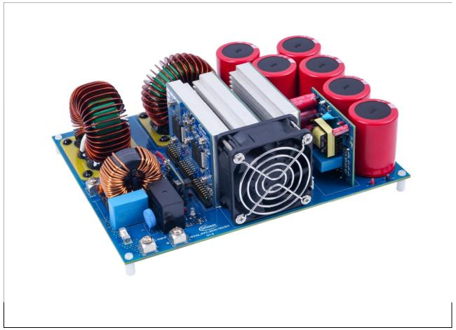
Figure 1 EVAL-1EDSIC-PFC-5KW: 5kW interleave totem pole PFC
