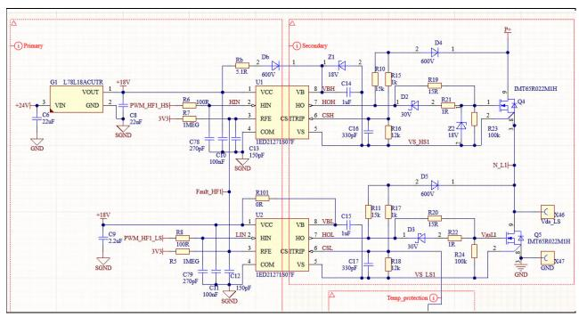
Figure 11 High frequency bridge
