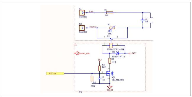
Figure 14 Inrush circuit
