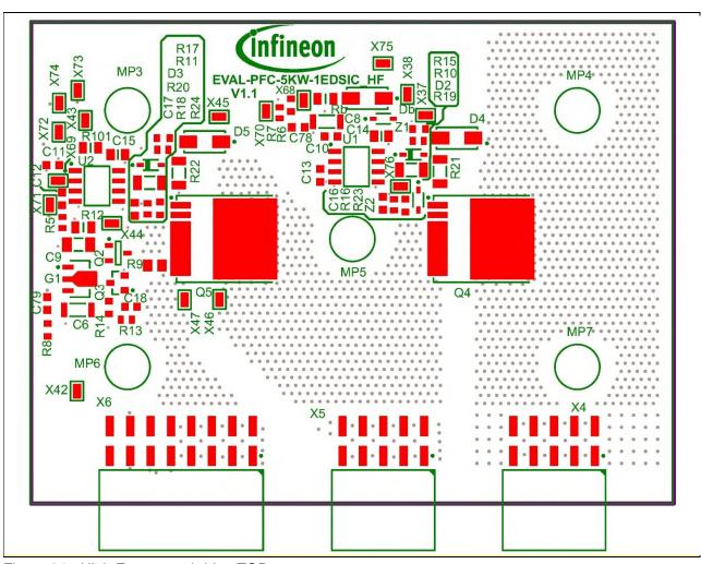
Figure 34 High Frequency bridge TOP
