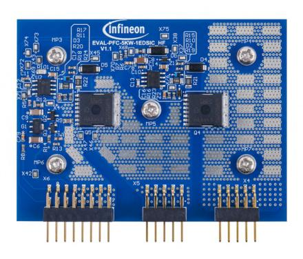
Figure 5 high-frequency 22mΩ 650 V CoolSiC™ (IMBG65R022M1H) in a PG-TO263-7 pin package, with 1ED21271S65F
