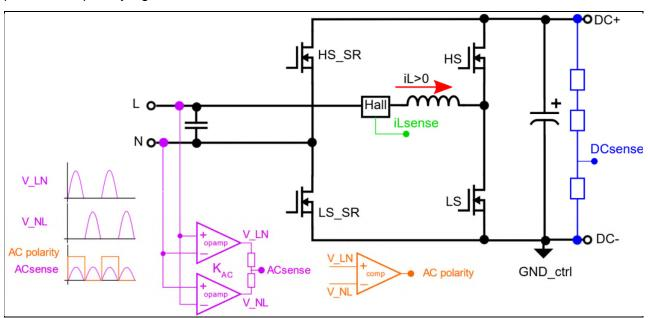
Block diagram of the sensing circuitry required for bidirectional totem-pole control with Figure 17 XMC™ and control reference in the AC rail in series with the PFC choke
