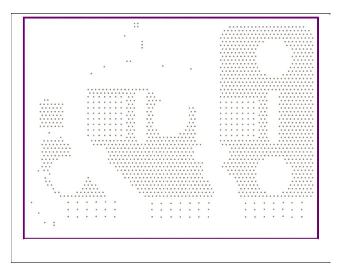
Figure 37 Return Path: Low Frequency Half Bridge Board BOTTOM
