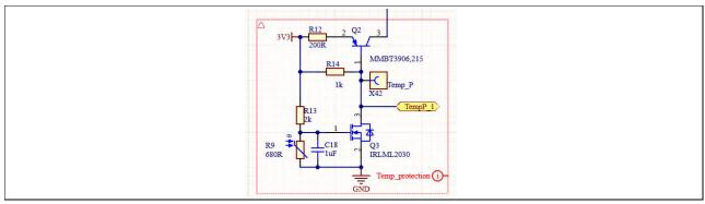
Figure 13 Temperature Protection circuit
