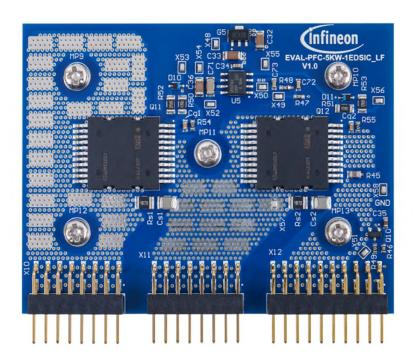
Figure 6 Return path board (low-frequency bridge) (50/60Hz), 10mΩ 600 V CoolMOS™ S7 (IPQC60R010S7) in a PG-HDSOP-22 package, with 2ED2182S06F gate driver
