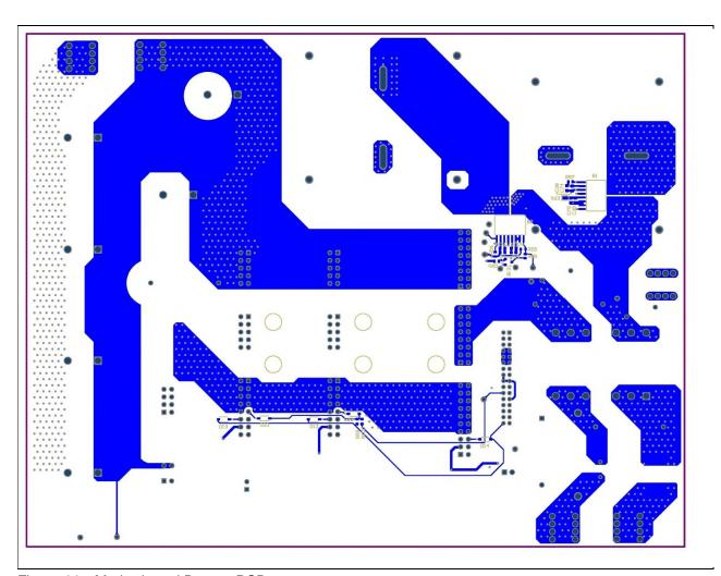
Figure 30 Motherboard Bottom PCB
