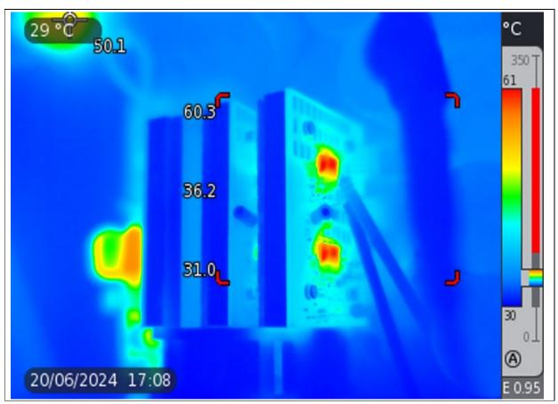
Figure 45 Board thermal characterization at Vac 180V and Vdc 400V, full load
