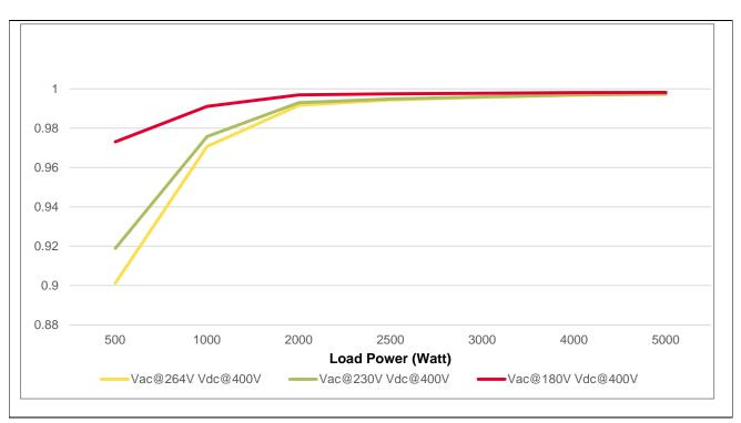
Figure 39 Power factor at different AC voltage
