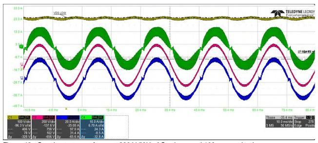
Figure 42 Steady-state waveforms at 230 V 50Hz AC voltage and 100 percent load
