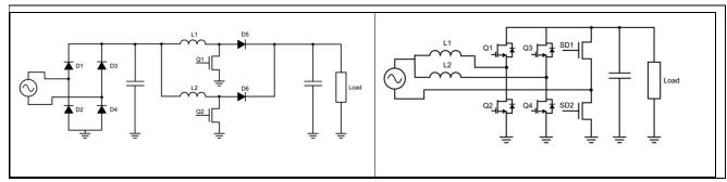
Figure 2 Interleaved Boost Totem Pole on the left and Interleaved Totem-Pole on the right
