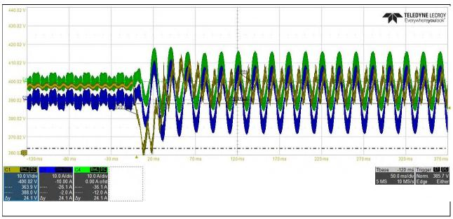
Figure 43 Load from 50 to 100 Vac@220V Vdc@400V
