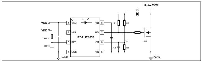
Figure 8 Over-current protection with de-sat detection circuit
