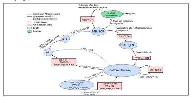
Figure 15 Totempole state machine for the interleaved 5kW PFC operation
