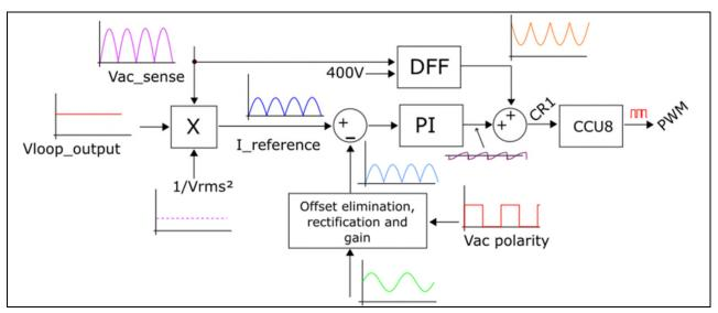
Figure 18 Current loop structure with duty cycle feed-forward and the required current manipulation
