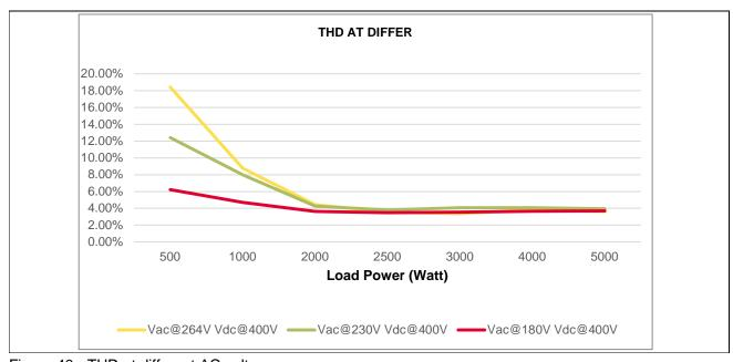
Figure 40 THD at different AC voltage
