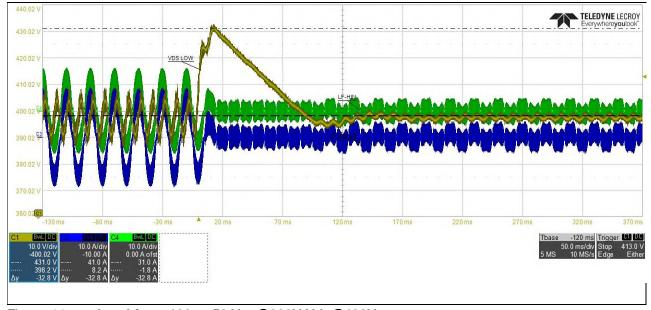
Figure 44 Load from 100 to 50 Vac@220V Vdc@400V
