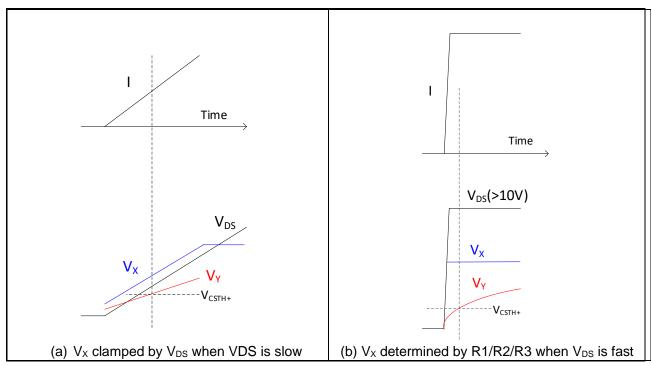
Figure 9 1ED2127 de-sat circuit
