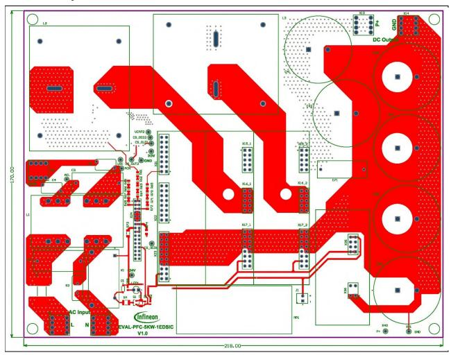
Figure 29 Motherboard TOP PCB
